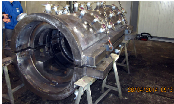
Fig. 7 Pressure-resistant recipient with welded flanges
