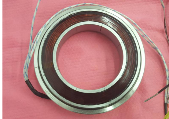
Fig. 2: Photograph of thrust bearing showing the segmented poles and the coil winding
