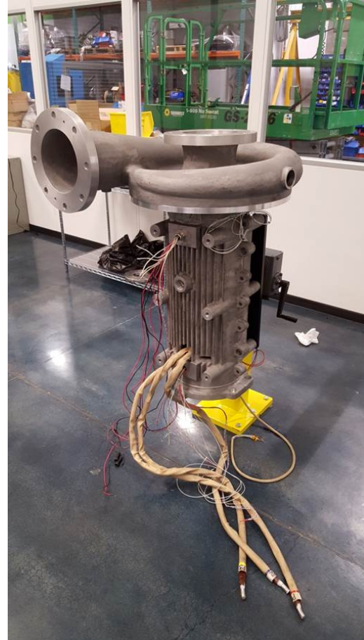
Fig. 2: Turbo-aerator core machine assembly showing the assembled aerator volute, motor casing, AMB power cables, and motor leads.
