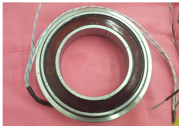
Fig. 4: Photograph of the thrust stator showing the segmented poles and the coil winding.
