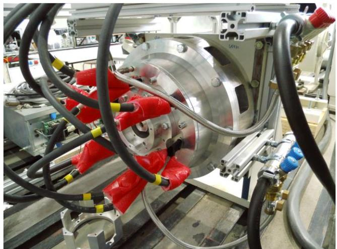
Figure 14 Flywheels system on the test bench
