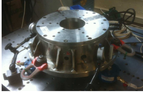
Fig. 4 Actuator force response characterization test rig. The disk (floator 2) is connected rigidly to the frame 1 through 7 and 8, while the stator of the actuator 3 is connected to the load cells 4 thanks to 9, 10 and 11. Conversely, the two parts of the stator are fixed together through an annular spacer 9 that guarantees the distance between them. A position sensor 6, fixed to the stator and targeting to an extension of the disk 5, allows the measurement of the relative deformation.
