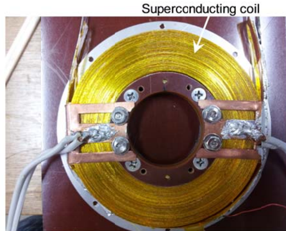
Fig.3 Superconducting coil for suspended object A copper coil is installed inside the superconducting coil. In the experiments the superconducting coil and the copper coil are in a liquid nitrogen container.
