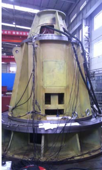
Fig.1 The test rig of helium circulator of HTR-PM
