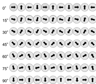
Fig. 4 Conceptual diagram of seven analysis patterns depending on the synchronized rotational angle of all cylinder-shaped permanent magnets.
