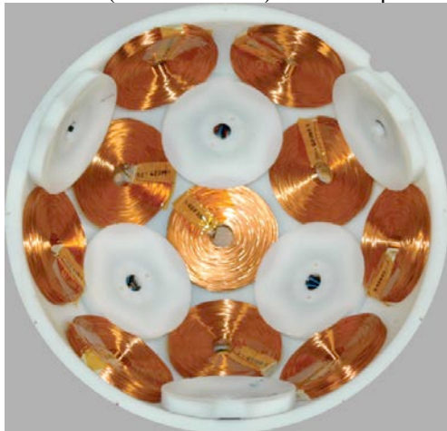
Figure 2 Stator (ironless) for a spherical momentum rotor of 20 cm diameter. Half of the 20 stator coils, arranged at the vertices of a regular dodecahedron, can be seen. The rotor consists of a sphere with Nd-Fe-B magnet shells in a 4 pole-pair arrangement, oriented as the vertices of a cube.
