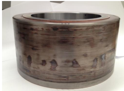
Figure 15. Stator pad deposits on landing sleeve after 7600 rpm landing test.
