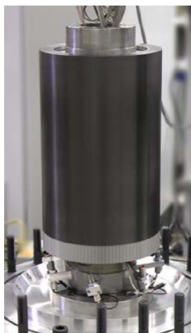
Figure 3. Picture of the rotor on the stator during system assembly
