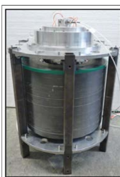
Figure 2. A magnetically levitated flywheel with composite shell has been designed and constructed. Picture from [15]
