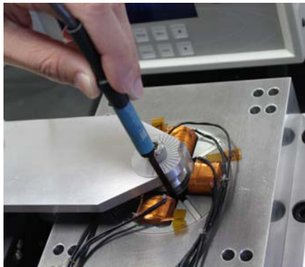
Figure 11. Fabricated magnetic bearing and flux density measurement
