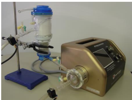
Figure 4. Preclinical maglev centrifugal blood pump system using Type 1 magnetic bearing and magnetic coupling mechanisms
