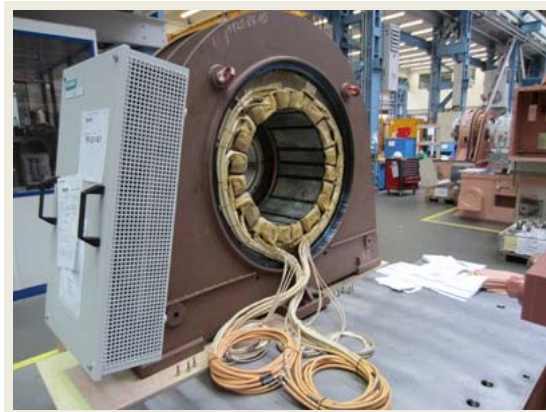
Figure 1. Radial magnetic bearing of the prototype motor from the SIMOTICS Active Magnetic Bearing series.
