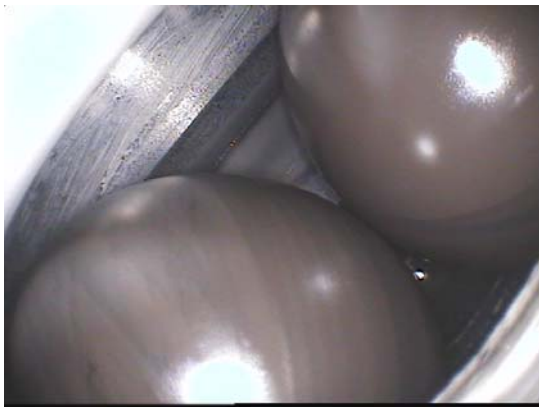
Figure 9. Optical endoscopic examination of the bearings after the 100sec drop at different regions of the bearing did not show any worrying amount of wear.
