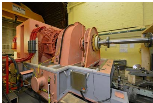
Figure 3. Motor setup during the landing tests with the original coupling and coupling spacer mounted on the EDE side to provide axial guidance.
