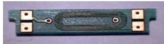
Figure 1. A sample of a HF transformer made of a PCB
