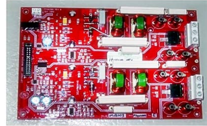
Figure 3. Existing Zephyr Amplifier PCB.
