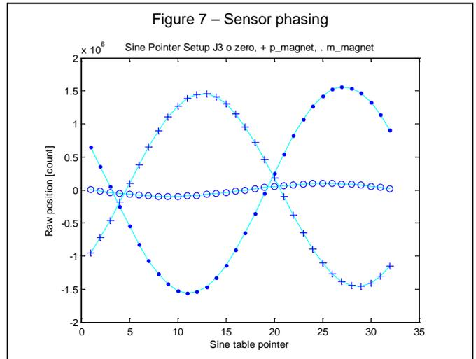
This figure also shows that the sensor has good sensitivity without risk of saturation. Time for the de-levitated sensor calibration (which was performed using dial gauges) was 24 minutes for the 5 individual axes and 9 minutes for the 2 radial bearing planes.
