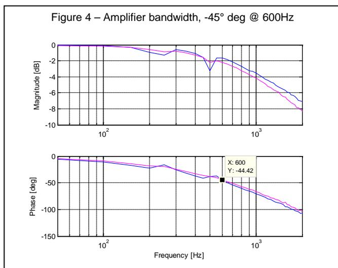
Next, the levitation script was used by the remote engineer to levitate and fine tune each axis in turn using initial calibration and loop shaping schemes from rotor dynamic analysis. The goal of this step is to achieve a soft suspension to allow better centering of the rotor. For this machine, we used remote manual adjustment of the controller terms to stabilize the suspension, but as discussed below, we plan to automate the heuristics used manually to achieve a stable suspension.
