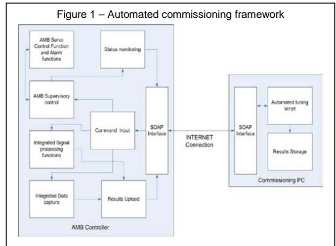
Automated commissioning works in parallel with the existing browser based AMB display system. The display system remains connected over the same network connection as the automatic commissioning tools and provides additional opportunities to monitor the commissioning progress. For remote commissioning it is occasionally helpful to exchange digital photographs of the bearing installation or arrange a video conference with a mobile camera to examine more details.
