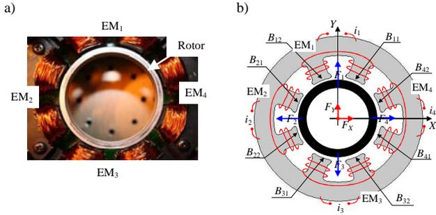
Figure 2. AMB with four actuators, smooth poles, and a ring-type rotor in the slim configuration: AMB and rotor thickness is 10mm
