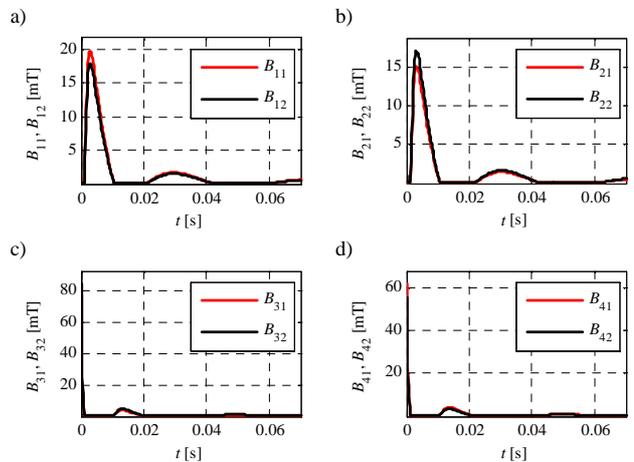
Figure 4. Magnetic flux density measured at every AMB pole (refer to Fig. 2) in the stabilisation task (Fig. 3).
