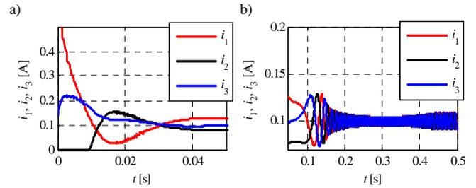
Figure 7. Control signals (coil currents) applied at the start-up and stabilisation phases under external rotary excitations
