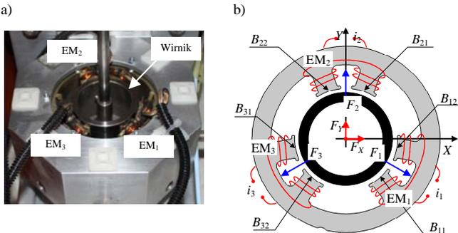
Figure 5. AMB with three electromagnets: a) prototype; b) model.
