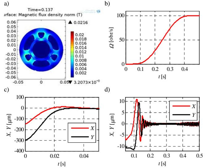
Figure 6. Distribution of magnetic flux density (a); rotor velocity profile (b) and rotor displacement (c) time diagrams: start-up (d) and stabilisation phase at rotations (e).
