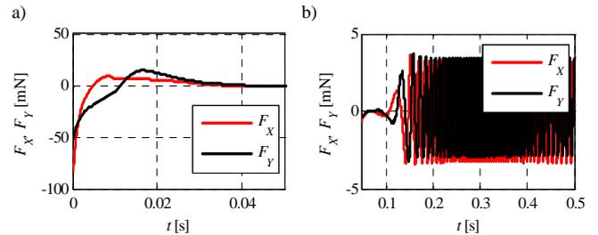
Figure 8. Calculated electromagnetic forces obtained at the start-up (a) and stabilisation (b) phases under external rotary excitations
