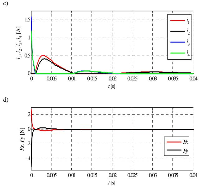
Figure 3. The simulation results of the stabilisation task - distribution of magnetic flux density (a); rotor displacement (b); coil currents (c) and electromagnetic force components (d).
