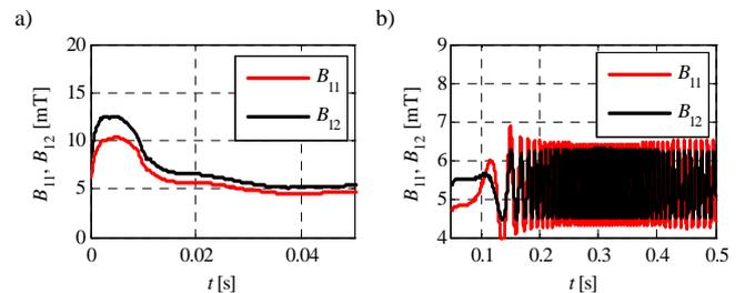
Figure 9. Measured magnetic flux density at EM1 poles, collected at the start-up (a) and stabilisation (b) phases under external rotary excitations
