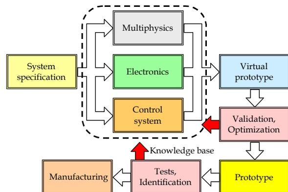
Figure 1. The proposed interdisciplinary design approach according to which the virtual prototype is being developed and studied
