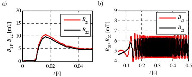
Figure 10. Measured magnetic flux density at EM2 poles - collected at the start-up (a) and stabilisation (b) phases under external rotary excitations.
