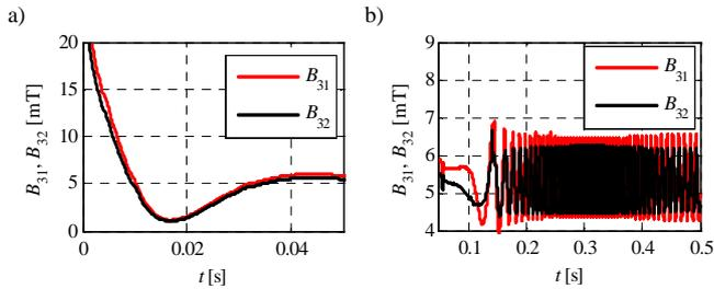
Figure 11. Measured magnetic flux density at EM3 poles - collected at the start-up (a) and stabilisation (b) phases under external rotary excitations.
