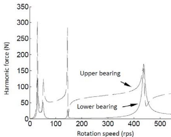
Figure 6. Harmonic response of the rotor.
