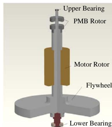
Figure 1. The structure of the Flywheel I rotor.
