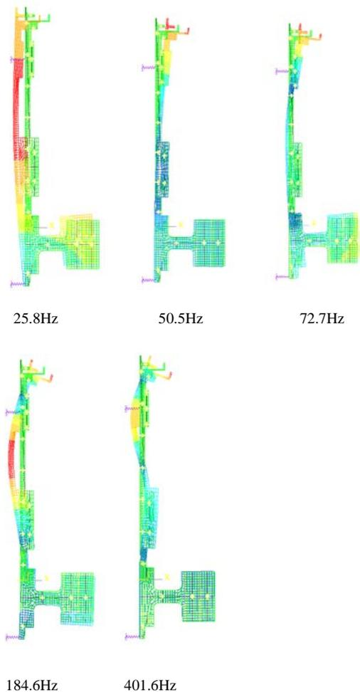
Figure 4. Vibration modes of the flywheel rotor.
