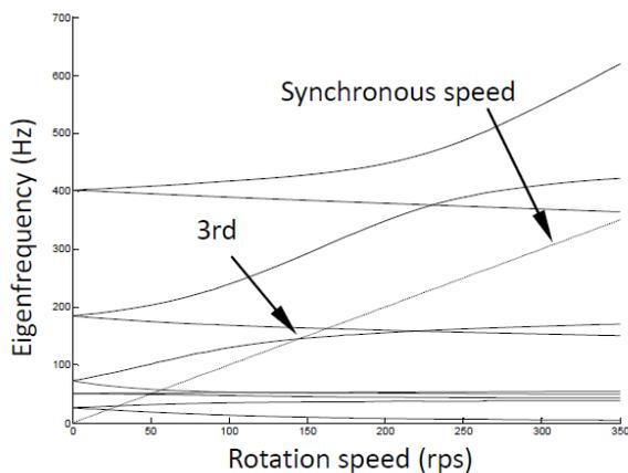
Figure 5. Campbell diagram for the rotor.
