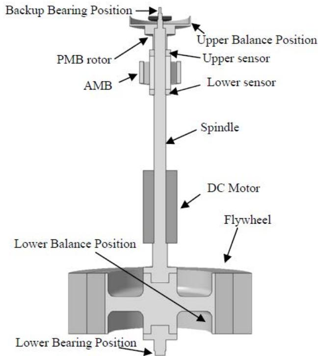
Figure 2. The structure of the Flywheel II rotor.
