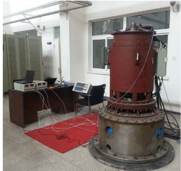
Figure 1. The structure and picture of the helium blower rig
