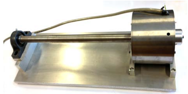
Figure 13. Laboratory setup of the homopolar three phase AMB.
