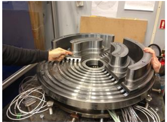
Figure 12. Reluctance type bearing with electrodynamic damper.
