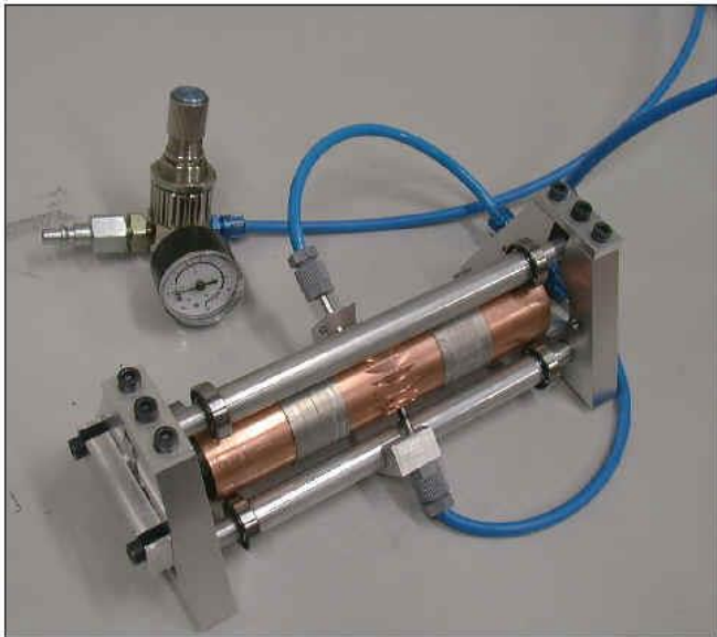
Fig. 10. Bleulers and Sandtner's test rig with air turbine and homopolar bearings.
