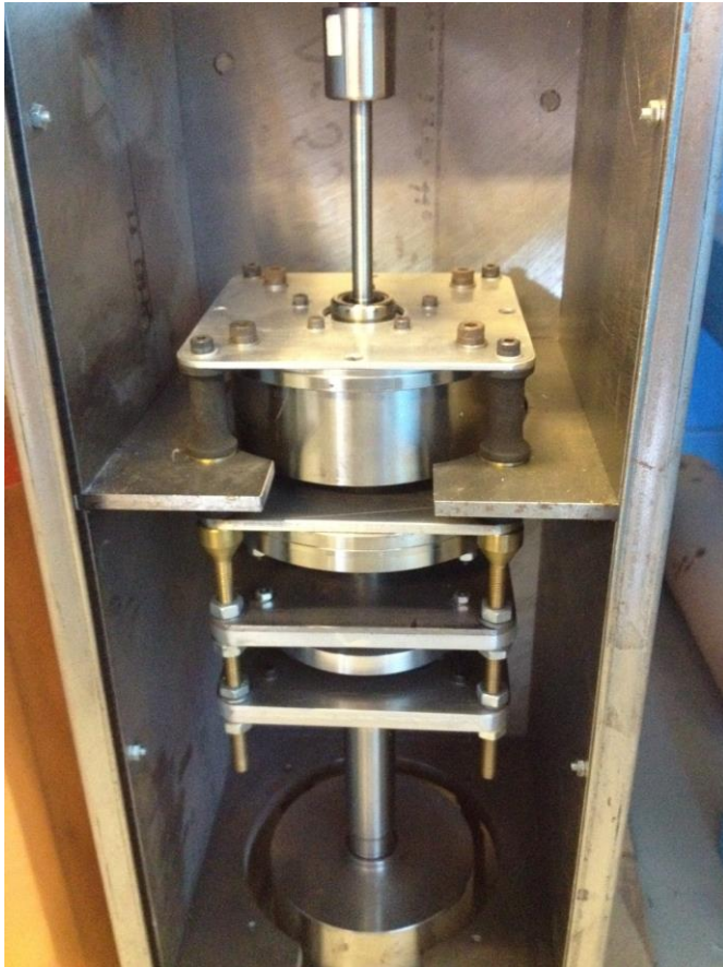
Figure 6. Prototype with heteropolar bearings designed by the author at SKF in 1990.
