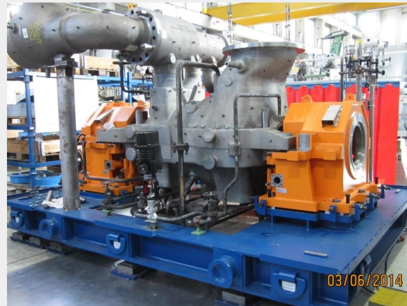
Prototype steam turbine during manufacturing in Goerlitz
