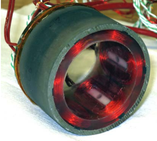
Figure 10. Experimental setup stator part. Air gap winding (epoxy resin bonded) with stator back iron.
