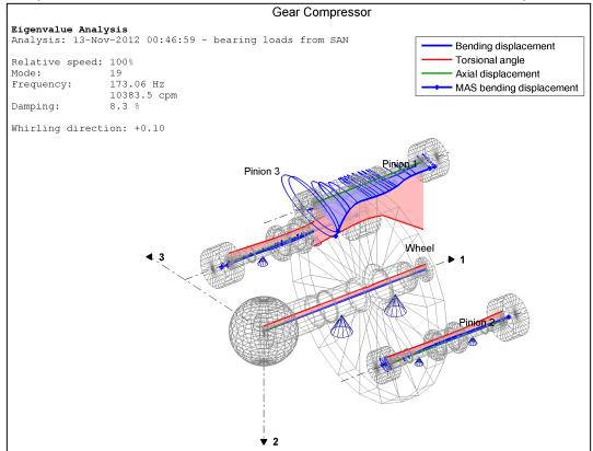
Coupled lateral torsional axial analysis of systems with gears
