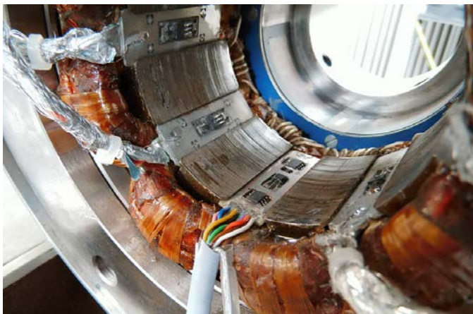
Figure 10. Sensors mounted at the test bearing. The lower sensor is the new version.
