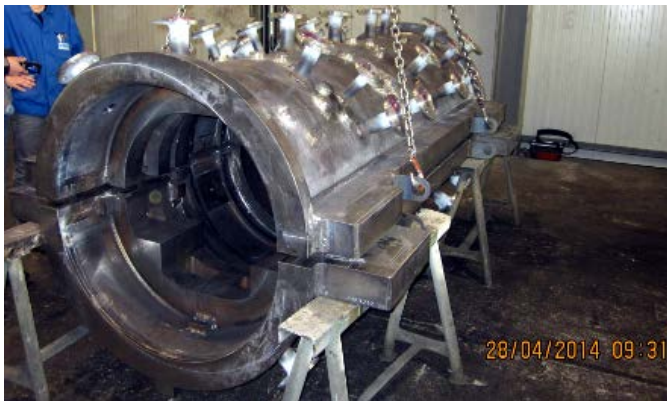
Figure 3. Pressure-resistant recipient with welded flanges
