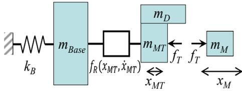
Figure 2. Dynamic model for reaction force compensation mechanism of moving magnet type
