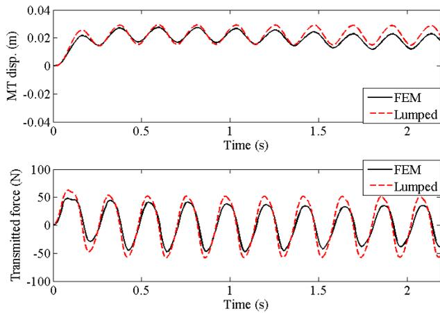
Figure 5. Comparison of Lumped and FEM analyses
