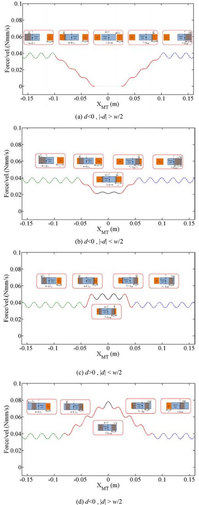
Figure 3. Eddy current force variation according to the magnet track position
