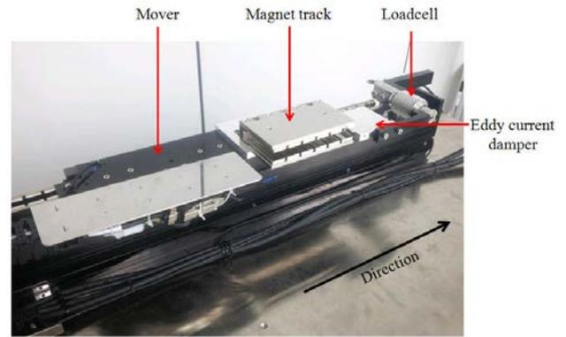
Figure 6. Experimental set-up
