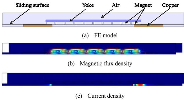
Figure 4. FEM analysis of the ECD with moving magnet track
