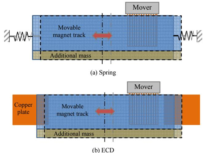
Figure 1. Passive reaction force compensation mechanisms
