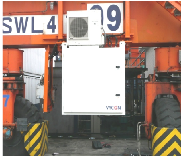
Figure 5. Vycon REGEN Installed on RTG
