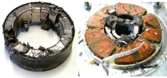
Figure 3: Rotor failure due to centrifugal forces at high speeds
