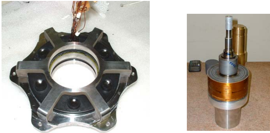
Figure 11 Radial, Homopolar Magnetic Bearing and Rotating Assembly
