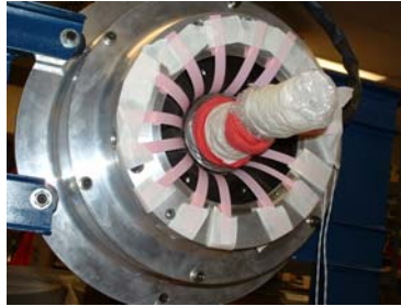
Figure 14 Radial Bearing Centered for Inductance Measurement
