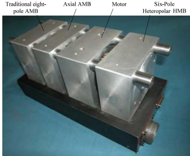
Figure 12: Five freedom magnetic bearing test-bed
