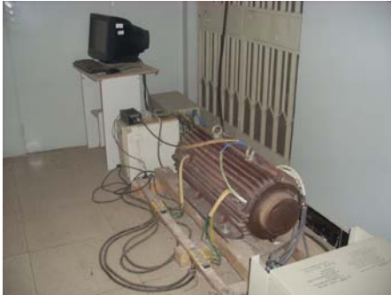
Figure 8: View of magnetic suspension blower prototype
