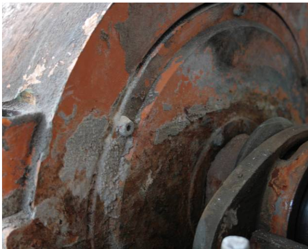
Fig. 3: Deposits and pitting corrosion on the bearing housing
