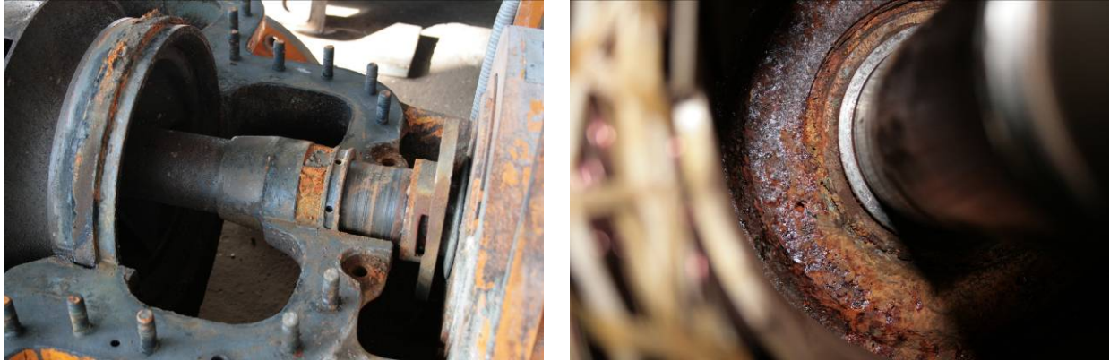
Fig 6: Primary and secondary radial touch down bearings
