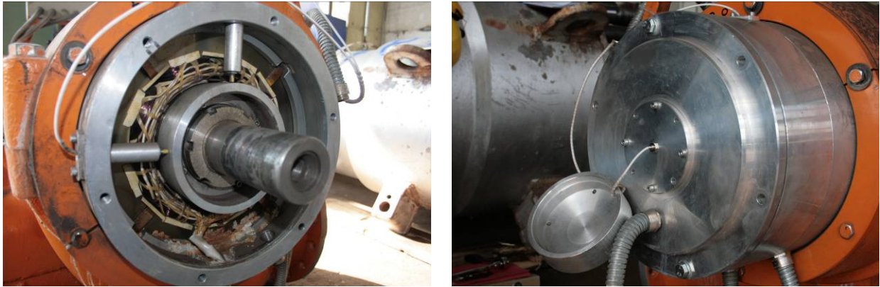
Fig. 4: DE-sited radial measuring system for shaft position and axial position sensor
