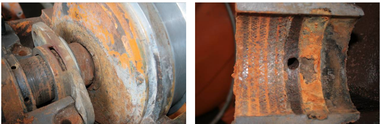
Fig 7: Wear in the area of the shaft seals at the shaft sleeve and in the pump cover
