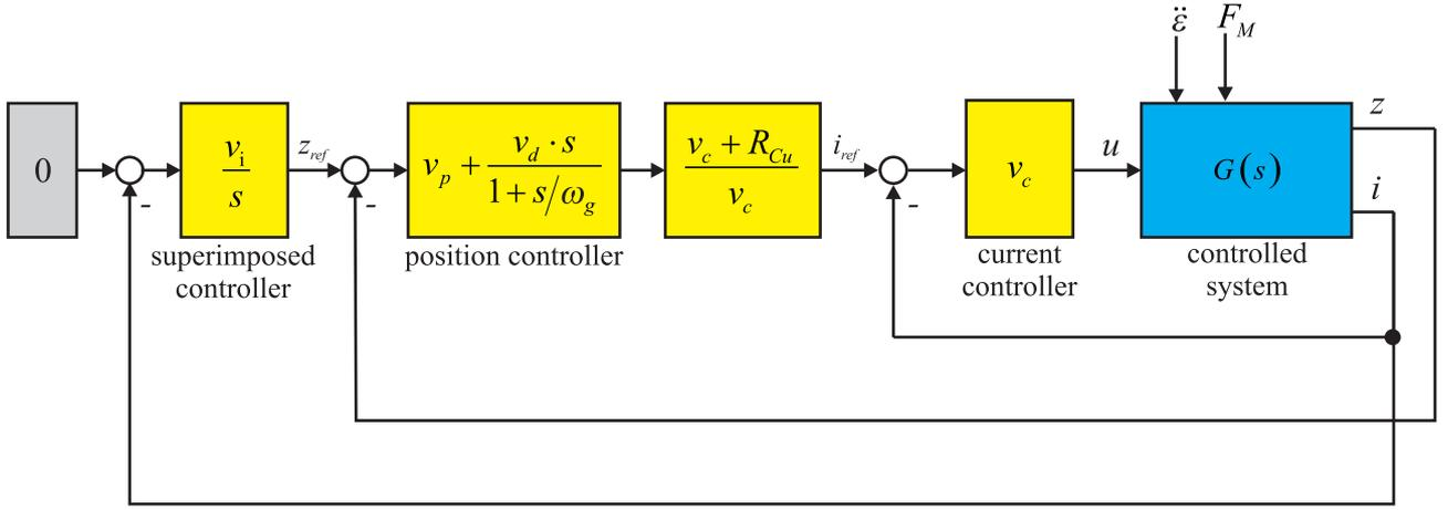
Fig. 3. Control structure used for the stabilization of the axial degree of freedom
