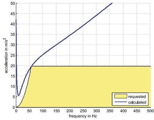
Fig. 5. Stabilizable accelerations of the housing for an optimized set of controller parameters (rigid stator–housing connection)
