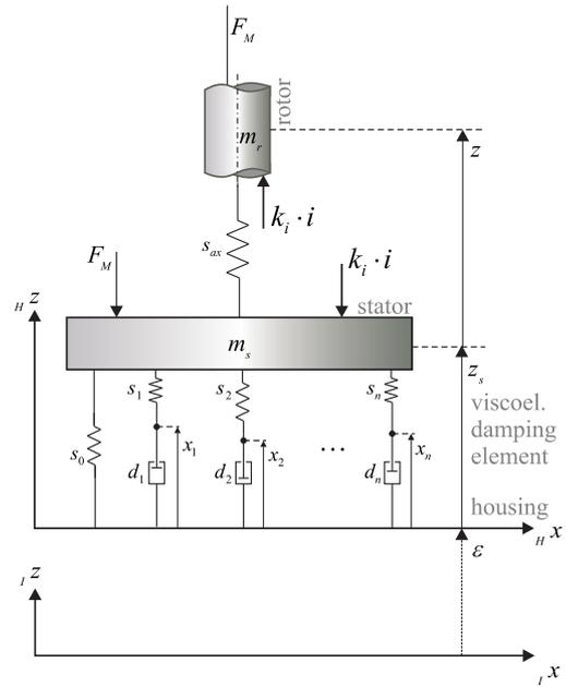
Fig. 2. Schematic representation of the vibrating bodies and the forces acting in axial direction. The viscoelastic damping element is modeled by a generalized Maxwell model.
