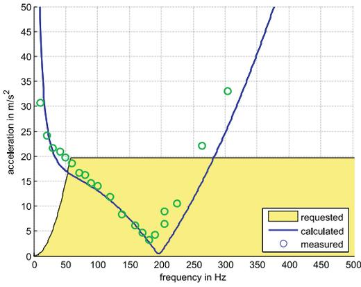
Fig. 4. Stabilizable accelerations of the housing for a freely chosen set of controller parameters (rigid stator–housing connection)
