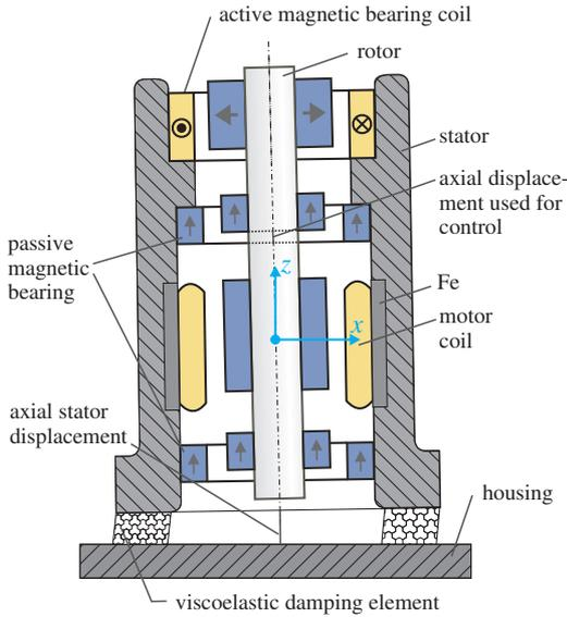
Fig. 1. Schematic representation of the entire assembly. The stator also performs axial deflections due to the elastic mounting.
