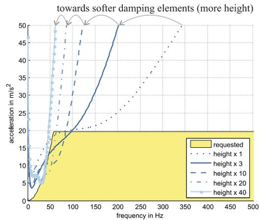
Fig. 7. Stabilizable accelerations of the housing for varying axial stiffness of the damping element. The controller parameters are optimized for each configuration.
