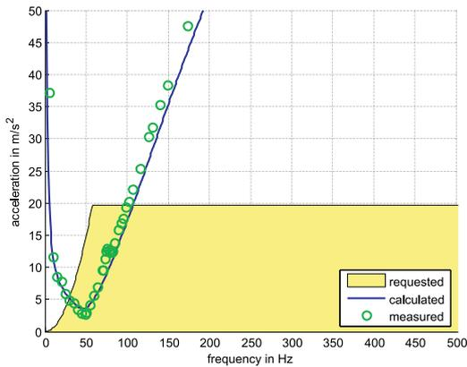
Fig. 6. Stabilizable accelerations of the housing for an optimized set of controller parameters. The requested transfer function cannot be achieved with the used damping element.
