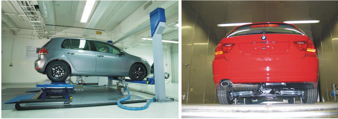
Fig. 1: Car vibration test rigs with magnetic reluctance actuators: Twin-shaker configuration (left), quad-shaker configuration (right, actuators located on intermediate floor). Pictures courtesy of VW AG and BMW Group.
