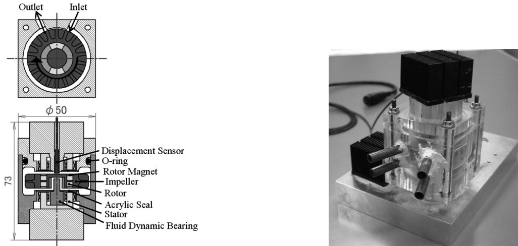
Fig. 4 Structure of push-pull-type pump
