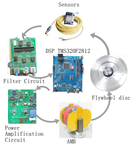
Fig.5 Frame of DSP control system
