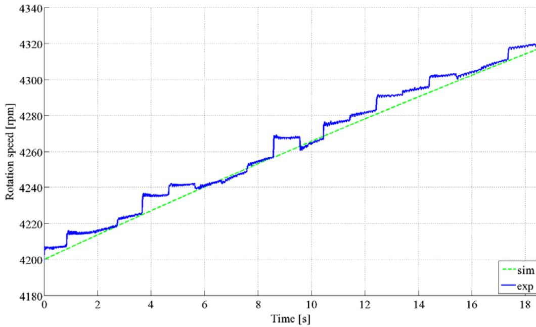
Fig.6 Comparison simulations and experiments (flywheel rotation speed)
