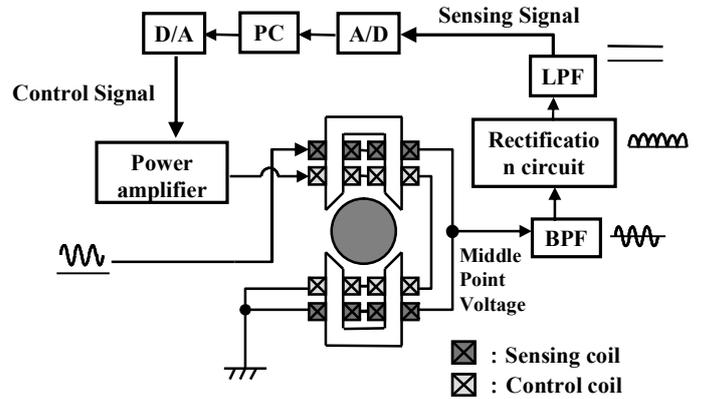
FIGURE 4: Self-sensing system
