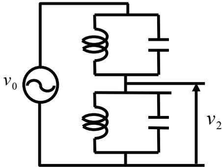
FIGURE 2: Resonant circuit for sensing
