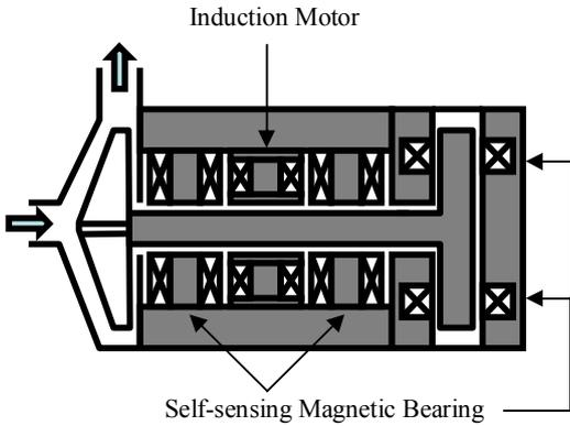
FIGURE 1: Structure of a liquid nitrogen pump
