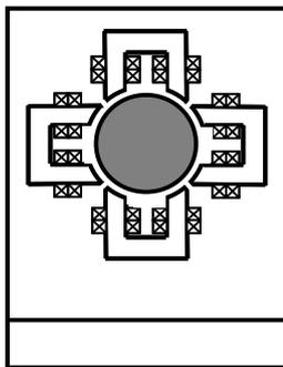
FIGURE 11: Structure of electromagnet for two axis control
