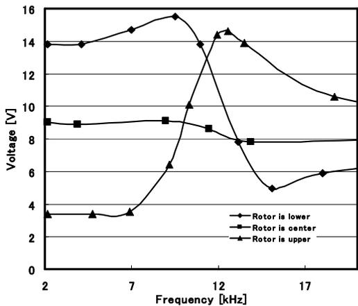
FIGURE 3: Change of middle point voltage to the frequency
