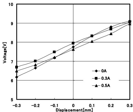
FIGURE 8: Middle point voltage (control current 0A, 0.3A, 0.5A)
