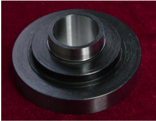
FIGURE 4: The workpiece finished using the active magnetic bearings spindle grinder
