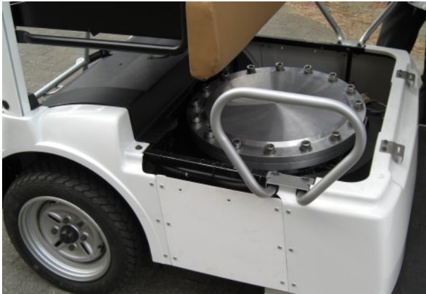
FIGURE 2: Flywheel attached to golf cart using gimbal mechanism
