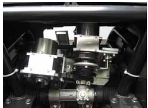
Figure 7: Modified front steering with steering by wire
