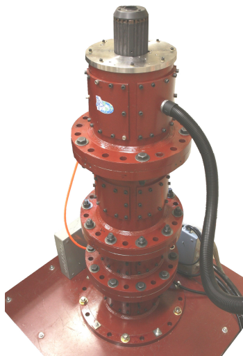
FIGURE 5: Vertical rotor test rig at SwRI facilities
