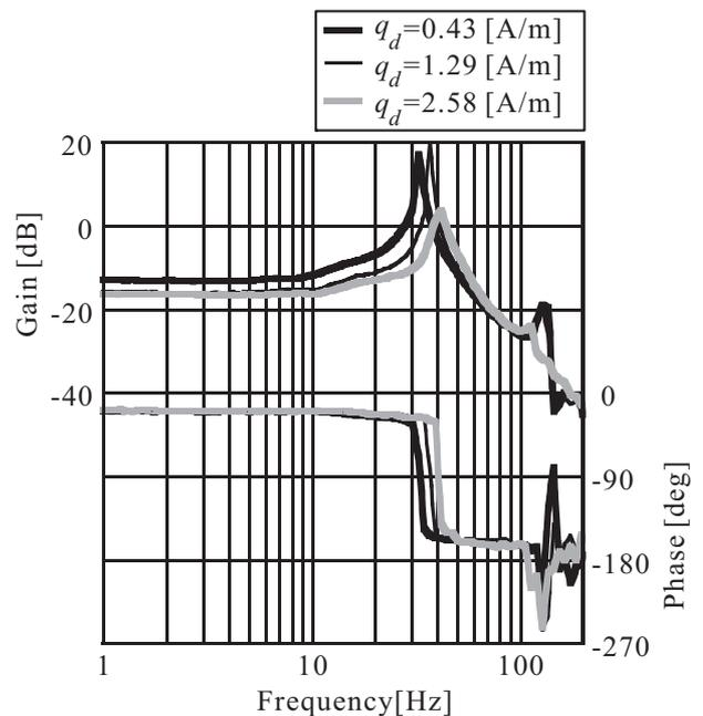
Fig.7 Frequency response of the R-unit 1.
