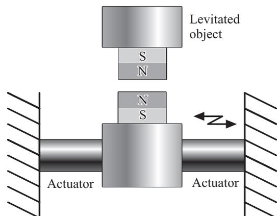
Fig.1 Concept of magnetic levitation system using the motion control of permanent magnet of support
