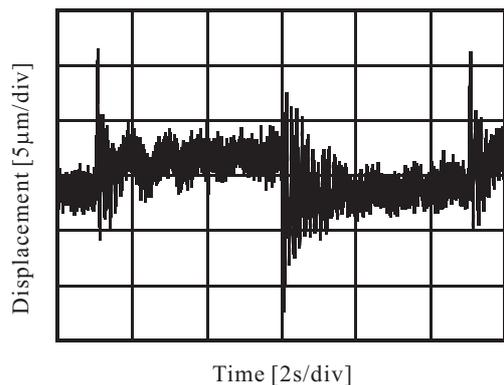
(a) Vertical displacement of the rotor
