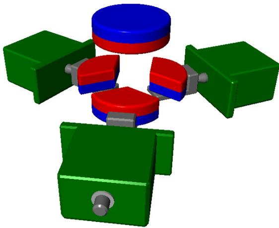
Fig.3 Schematic diagram of a levitation system with a three-segment permanent magnet of support for three-dimensional motion control.
