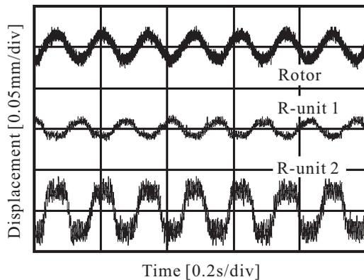
Fig.8 Movements of the rotor and the units when the lateral motion is stabilized
