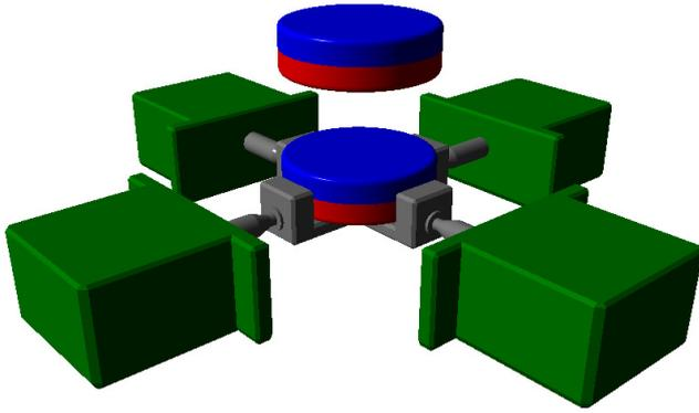
Fig.2 Schematic diagram of a levitation system with a single permanent magnet of support for two-dimensional motion control.
