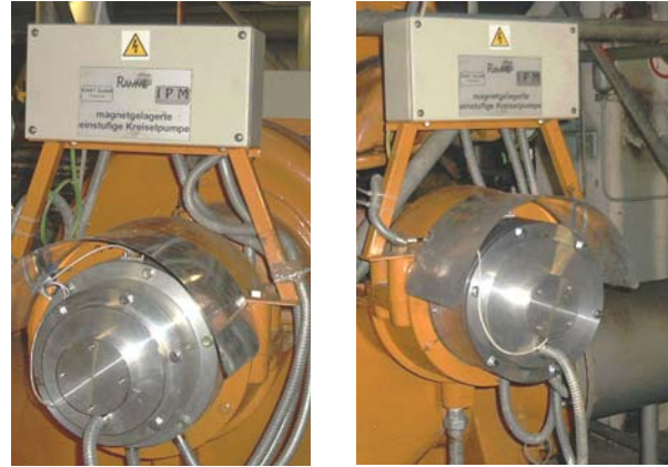
Fig. 6 Previous and new Axial Magnetic Bearing
