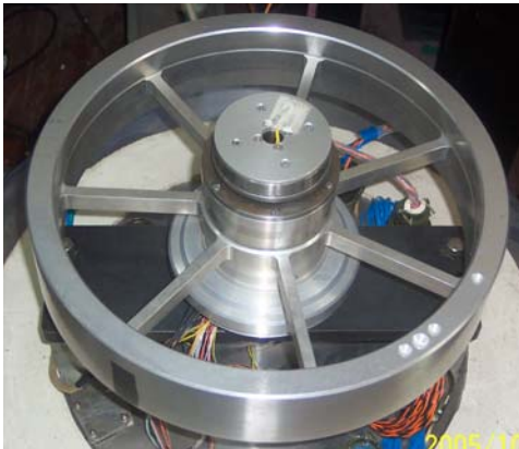
Fig. 10 The photo of 5-DOF MBRW system
