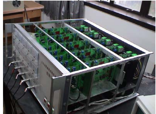
Fig.7 The outward appearance of system controller and the internal structure.
