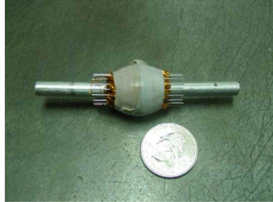
Figure 4: Stator Windings Before Forming
